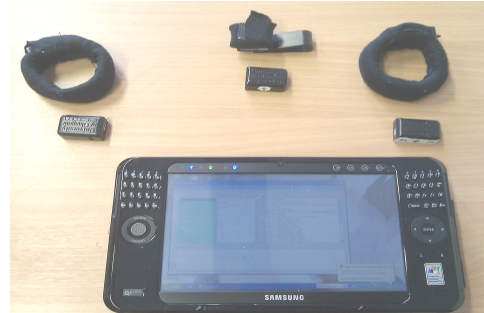
Figure 2. All the equipment used to interact with the Gesture RSS system. At the top, three JAKE sensor packs with two wristbands and one clip to attach the device to a user’s wrists and back of the collar. The sensors connected to the UMPC (carried in a rucksack) via Bluetooth.
