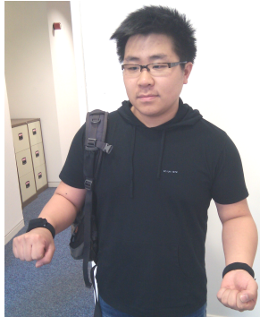
Figure 1. One participant using the system. A UMPC is in a backpack while two wrist bands contain sensors used for input. An additional sensor is worn on the back of the collar.
